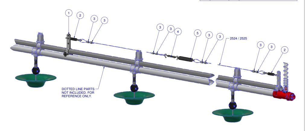
FAILURE TO USE 3/32" OR 2.4 MM O.D. 1 X 7 GALVANIZED CABLE WILL MOST LIKELY REQUIRE PERIODIC RE-TIGHTENING OF THE ANTI-ROOST SYSTEM AND/OR REPLACEMENT OF THE CABLE AND INSTALLATION ASSEMBLY HARDWARE.
