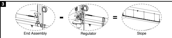
If the slope is greater than 75 cm / 30 in, reconfigure the system.
