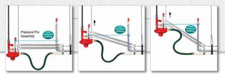
Regulator never needs adjustment. Pressure Pro at lowest possible position (horizontal) provides a minimum line pressure setting. As birds grow, elevating the regulator increases line pressure.
