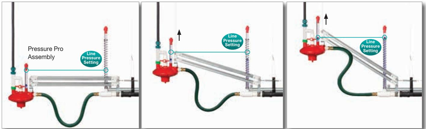
Regulator never needs adjustment. Pressure Pro at lowest possible position (horizontal) provides a minimum line pressure setting.
