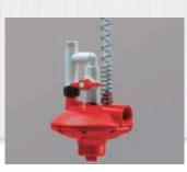
Flush Regulator Delivers high water volume at the low pressure required for no-spill drinking. Built-in flush valve makes for easy removal of sediment, biofilm and air.
