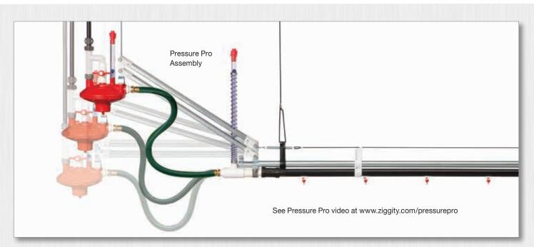
Pressure Pro makes drinker line pressure management so quick and easy that producers can more effectively manage litter conditions to improve bird performance, while also cutting costly management time from every production cycle.
