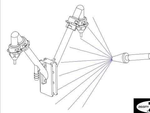
HIGH PRESSURE SPRAYING MAY CAUSE THE ELBOW SADDLE TO ROTATE AND WORK THEIR WAY OFF THE TL START GROW UNIT. NOTE ILLUSTRATIONS 1, 2 & 3.
