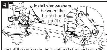
Install the remaining bolt, nut and star washers (25) from PN 2880. Important to install parts in same order as step 2.
