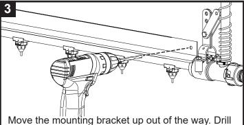
Move the mounting bracket up out of the way. Drill a hole at marked location using a 7 mm / 9/32 in drill bit.
