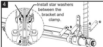
Install the bolt, nut and star washers (2x) from PN 2880. Important to install parts in same order as shown. Do Not tighten.
