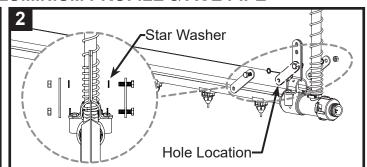
Install PN 2880 onto the regulator clamp in order as shown. Mark the hole location on the aluminium profile.
