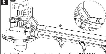
Install the remaining bolt and nut from PN 2880. Note: you will not use any star washers in this step. THIS PAGE INTENTIONALLY LEFT BLANK
