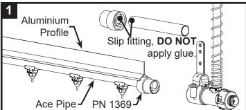
Sand the end of the ace pipe. Install PN 1369 onto the end of the ace pipe. Next install the end assembly onto PN 2235. Slip fitting, **DO NOT** apply glue.
