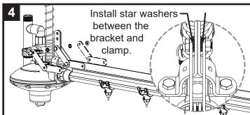
Install the bolt, nut and star washers (2x) from PN 2880. Important to install parts in same order as shown. Do Not tighten.
