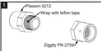
Wrap threads on Plasson 5212 Adapter - 32x25x3/4 in with teflon tape. Thread into PN 2759.
