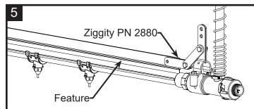
Align PN 2880 with the feature on the aluminium profile as shown. Mark the hole location on the aluminium profile. Drill a hole at marked location using a 7 mm / 9/32 in drill bit.
