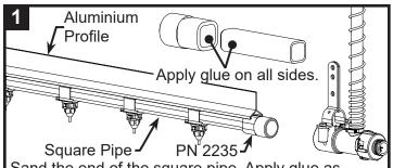
Sand the end of the square pipe. Apply glue as shown and install PN 2235 onto the end of the square pipe. Next install the end assembly onto PN 2235. Slip fitting, **DO NOT** apply glue.
