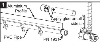
Sand the end of the PVC pipe. Apply glue as shown and install PN 1931 onto the end of the PVC pipe. Next install the end assembly onto PN 1931. Slip fitting, **DO NOT** apply glue.
