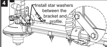
Install the remaining bolt, nut and star washers (2x) from PN 2880. Important to install parts in same order as step 2.
