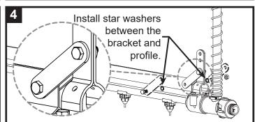
Install the remaining bolt, nut and star washers (2x) from PN 2880. Important to install parts in same order as step 2.
