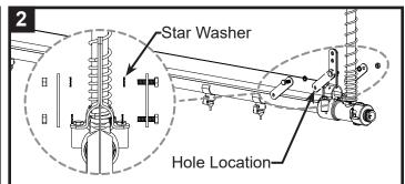
Install PN 2880 onto the end assembly clamp in order as shown. Mark the hole location on the aluminium profile.
