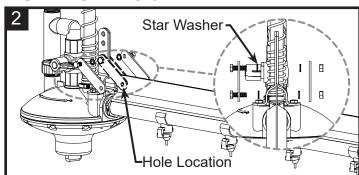
Install PN 2880 onto the regulator clamp in order as shown. Mark the hole location on the aluminium profile.
