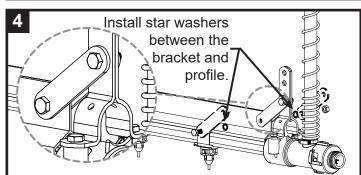
Install the remaining bolt, nut and star washers (2x) from PN 2880. Important to install parts in same order as step 2.
