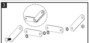
Attach PN 2880 (2x) together in order as shown. Do Not tighten. Leave loose to allow movement for future steps.
