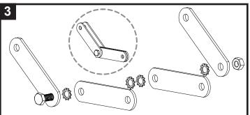
Attach PN 2880 (2x) together in order as shown. Do Not tighten. Leave loose to allow movement for future steps.
