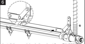
Install the remaining bolt and nut from PN 2880. Note: you will not use any star washers in this step.
