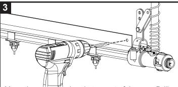
Move the mounting bracket up out of the way. Drill a hole at marked location using a 7 mm / 9/32 in drill bit.
