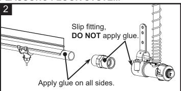
Sand the end of the pipe. Apply glue as shown and install assembled adapter.
