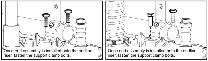
**Important:** Before fastening the support clamp fasteners, push or pull the endline riser assembly for correct gapping.
