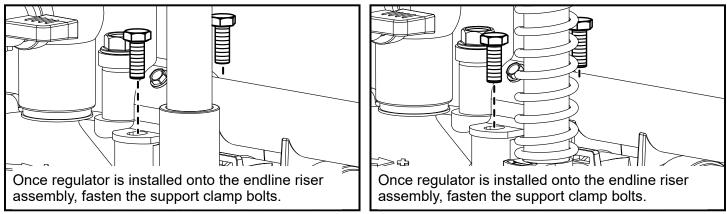
**Important:** Before fastening the support clamp fasteners, push or pull the endline riser assembly for correct gapping.
