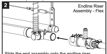
Slide the end assembly onto the endline riser. Make sure the end assembly is oriented correctly, as illustrated.
