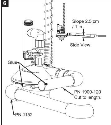
Glue PN 1152 onto PN 1900-120. Create a slope by angling the parts put together in step 5. (See side view)
