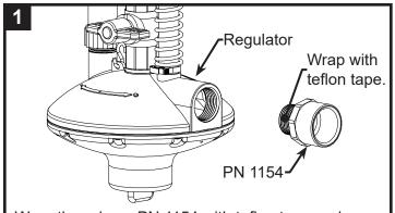
Wrap threads on PN 1154 with teflon tape and thread into the regulator.
