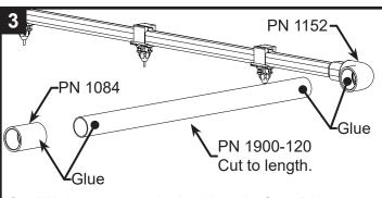
Cut PN 1900-120 to desired length. Glue PN 1900-120 into PN 1152. Glue PN 1084 onto PN 1900-120.
