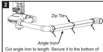
the sagging pipe with zip ties. Pull the zip tie tight and snip off the excess.
